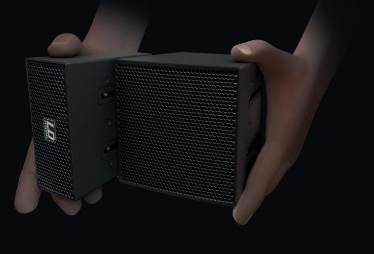
The innovative SmartLink<sup>®</sup> adapter forms the basis of the system. On top of that up to four Array Satellites can be effortlessly interconnected with the LD Systems-patented click mechanism: simply press the connection button, join the two modules by their guide rails and release the button to engage.
